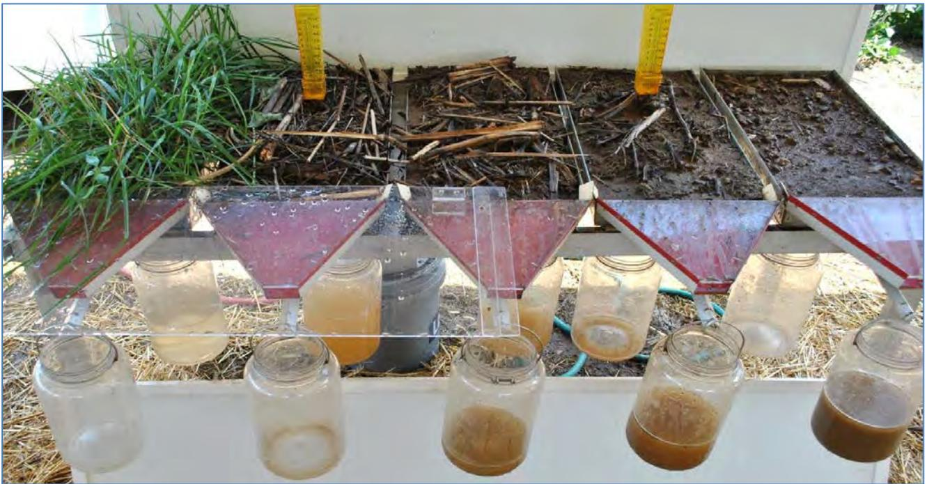
Above is a rainfall simulator that was on display at the conference. The jars out front were collecting the runoff. The jars beneath were collecting infiltration. The exhibit demonstrated the relationship of nurtured & neglected soils to runoff and infiltration.
