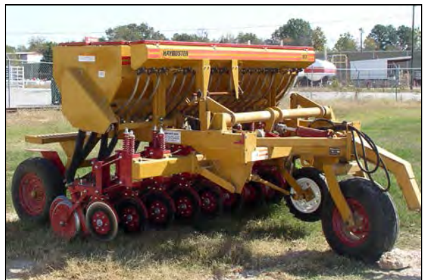
9-foot Haybuster no-till drill capable of planting legumes, grasses, and Native Grasses
